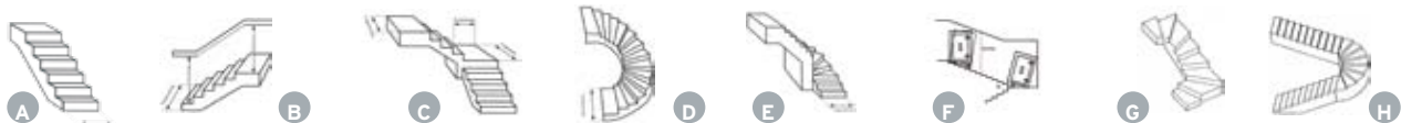
A straight stairs without a joist | B straight stairs with a joist | C 90° spiral staircase with platform | D 180° spiral staircase | E stairs with a 90° turning point | F 180° spiral staircase with platform | G stairs with a 2 x 90° turning point without a platform | H stairs with a 180° turning point
